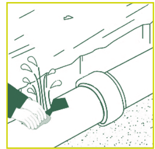
Apply the putty to the damaged area or leak and hold firmly in position without movement until set.
