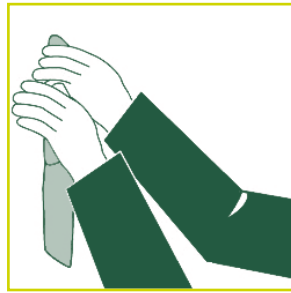
Apply the putty to the leak and hold firmly in position without movement until set
