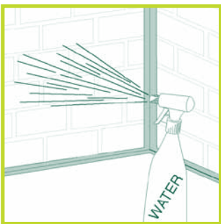
Well dampen surface with water ensuring no standing water.
