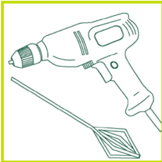
Rose bud paddle in electric drill 900rpm 1000w.
